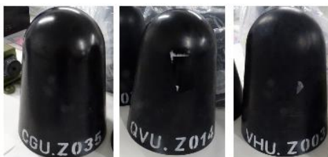
Marking pattern on the Borkan-2H nose tips: “CGU.Z035”, “QVU.Z014” and “VHU.Z003”
