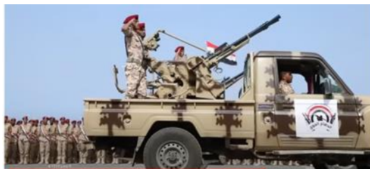
Figure 65.4. Mounted with ZU-23, 23mm twin-barrel air defence canon
