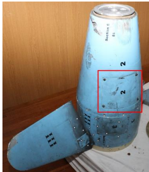
Figure 51.13. Access hatch in rear end section of a cruise missile used by Houthis in Sep- tember 2019 ARAMCO attacks in the KSA
