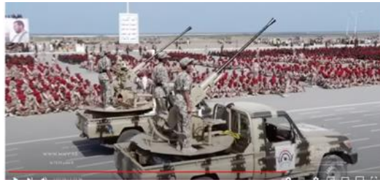
Figure 65.6. Mounted with 37mm twin-barrel anti-aircraft canon Type 65 or a variant of it
