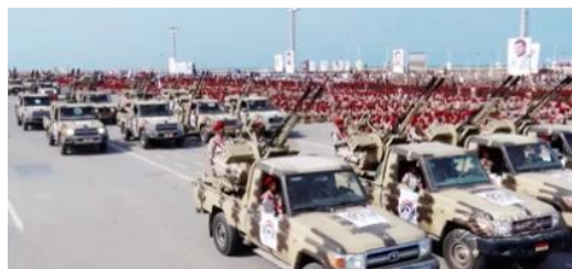
Figure 65.4. Mounted with ZU-23, 23mm twin-barrel air defence canon
